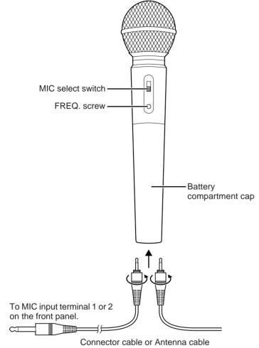
Two microphones are provided. One can be used as a wireless microphone, another one can be used as wireless or wired microphone.
