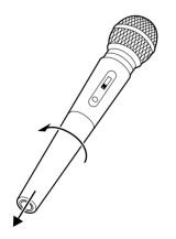
2 Insert 2 "AA/UM-3"-size batteries (provided) in the correct directions.
